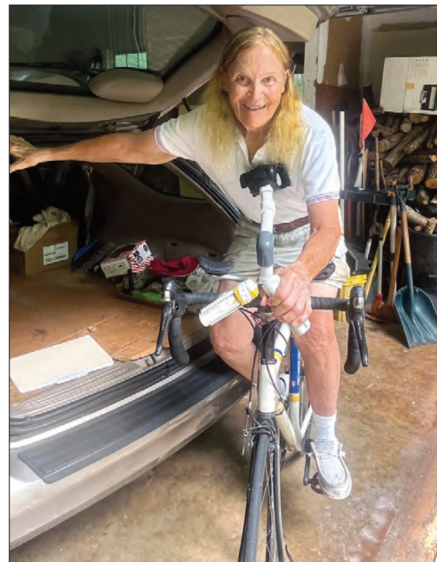
Narelle Kirkland demonstrates the Bicycle Chest Rest designed to relieve stress on the neck, back and arms while riding. A provisional patent has been obtained for the device.
