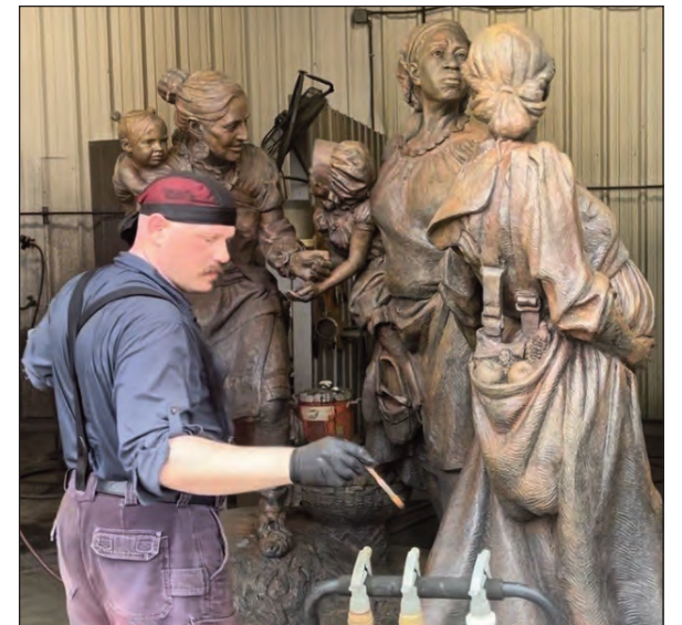
Following the dusting and the acid wash, the bronzing is meticulously applied to the sculpture.
