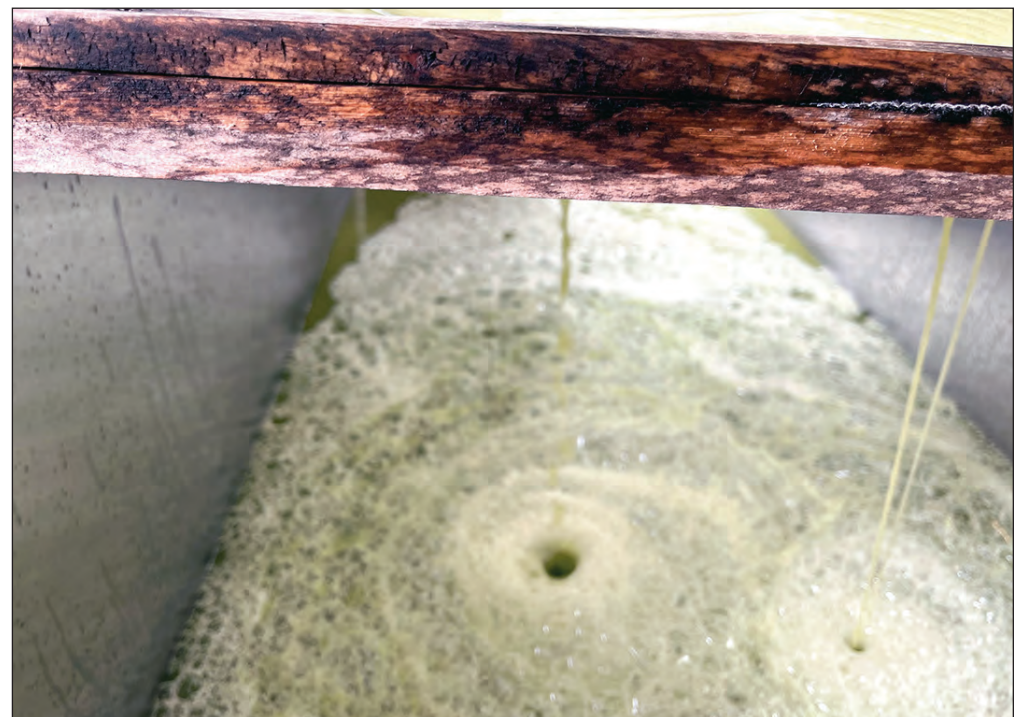
After the cane is pressed during the grinding process the juice is piped to a container that fills to ready for the boiling process.
