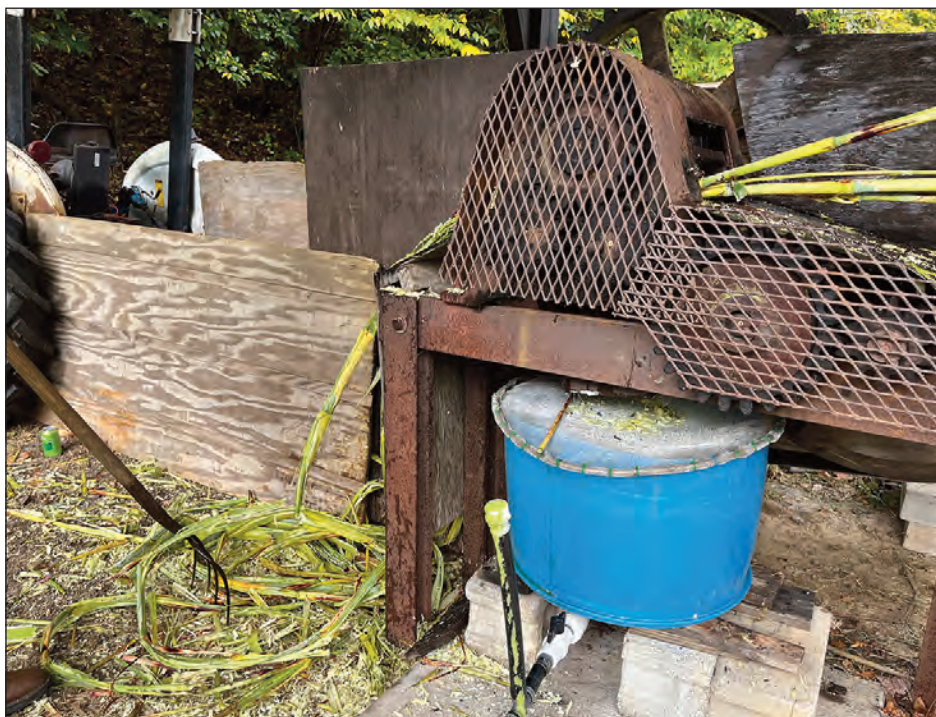
After the cane is pressed during the grinding process the juice is piped to a container that fills to ready for the boiling process.
