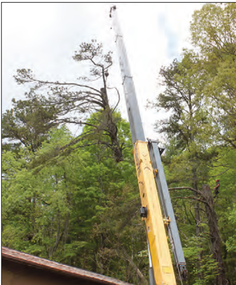
Recently the Lee Talley Tree Company took down a yellow pine tree that was threatening a nearby structure. Tree climber Brandon Elliott wielded the saw, first cutting the top of the tree, as crane operator Luke Cook guided it and two other sections to the ground where it was cut into 12-foot logs by Dustin Daves and Lee Talley. The process took about two hours. Photos by Betsey Gooder
