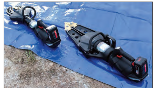
The new extrication equipment runs on a battery pack instead of needing a generator to operate.
