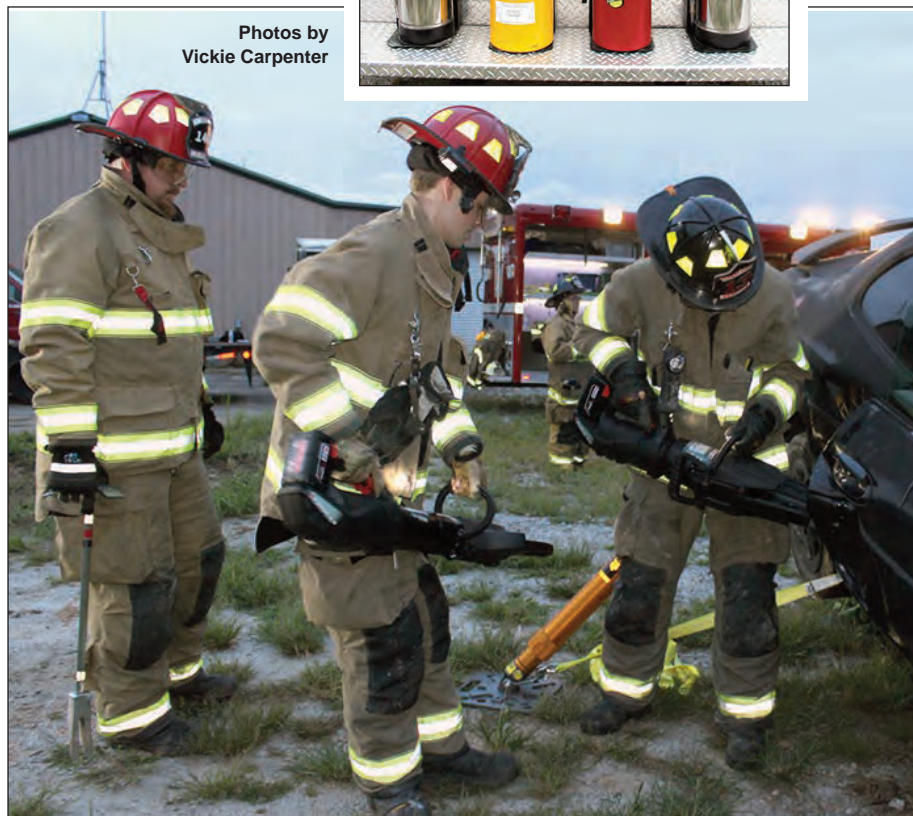
The new extrication equipment runs on a battery pack instead of needing a generator to operate.
