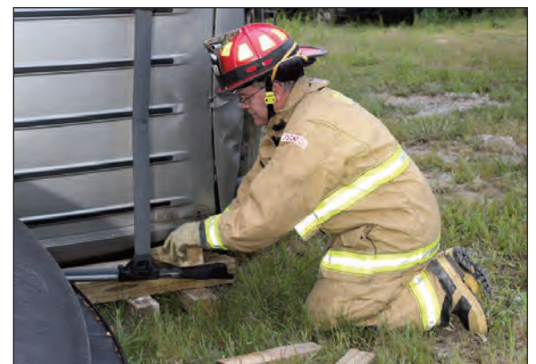
The new extrication equipment runs on a battery pack instead of needing a generator to operate.
